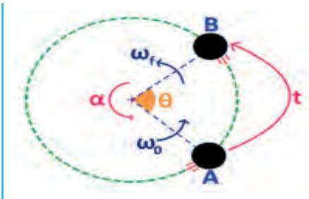
$$\begin{aligned}\omega_f &= \omega_0 + \alpha t \\ \omega_f^2 &= \omega_0^2 + 2\alpha\theta \\ \theta &= \omega_0 t + \frac{1}{2}\alpha t^2 \\ \theta &= \left(\frac{\omega_f + \omega_0}{2}\right)t \\ a_T &= r\alpha\end{aligned}$$
