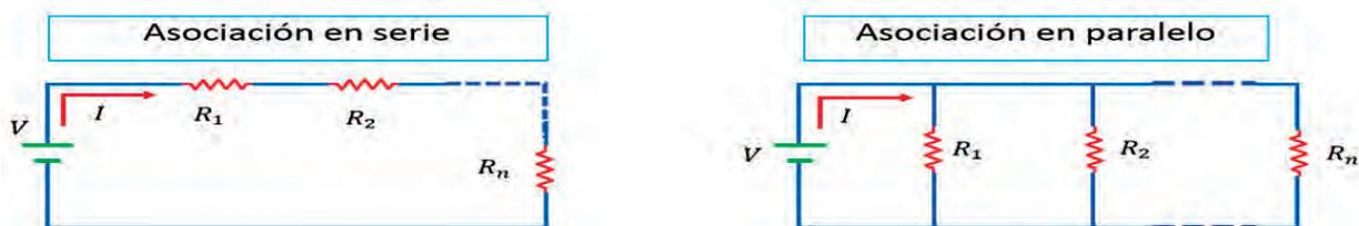
$$V_T = V_1 + V_2 + \dots + V_n$$
