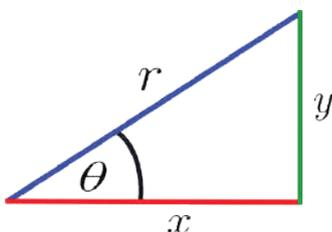
$$\begin{aligned} \text{sen}\theta &= \frac{y}{r} & \text{cosec}\theta &= \frac{r}{y} \\ \text{cos}\theta &= \frac{x}{r} & \text{sec}\theta &= \frac{r}{x} \\ \text{tg}\theta &= \frac{y}{x} & \text{ctg}\theta &= \frac{x}{y} \end{aligned}$$
