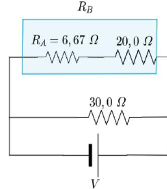
$$R_B = R_A + 20,0 \Omega = 6,67 \Omega + 20,0 \Omega = 26,67 \Omega$$
